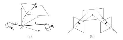
**Fig. 2.** (a) Plane and camera configuration. (b) The points are optimally corrected so that their rays intersect on the plane.
