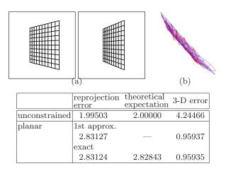
Fig. 5. (a) Simulated images of a planar grid taken from different places. (b) 3-D position of the reconstructed grid. Points reconstructed by planar triangulation (in blue) are on the specified plane, but those reconstructed by unconstrained triangulation [11] (in red) are not necessarily on it. The table below lists the reprojection error, its theoretical expectation, and the average 3-D reconstruction error.
