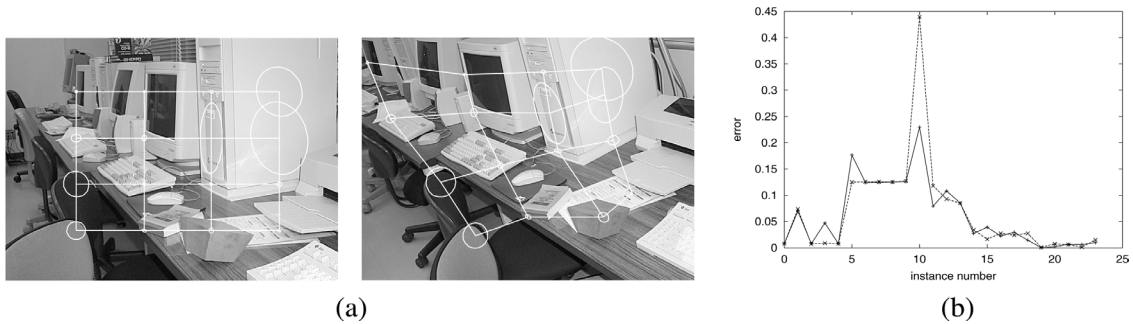
Fig. 6. (a) Covariance matrices and corresponding points. (b) Errors in the fundamental matrix computation using the covariance matrices evaluated from the gray levels (solid lines) and their default values (dashed lines). The numbers on the abscissa indicate individual instances.
