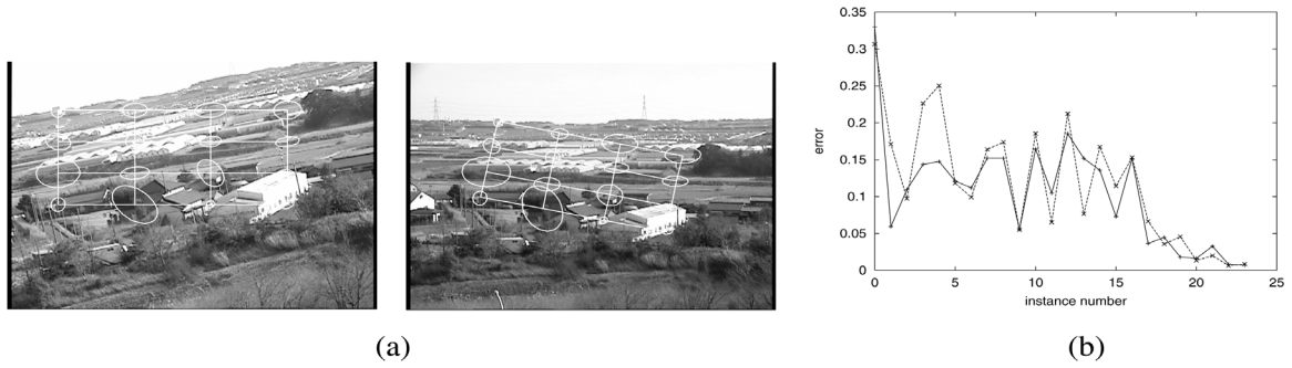
Fig. 5. (a) Corresponding points and their covariance matrices. (b) Errors in the homography computation using the covariance matrices evaluated from the gray levels (solid lines) and their default values (dashed lines). The numbers on the abscissa indicate individual instances.
