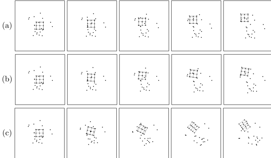
Figure 2: Simulated image sequences of 14 object points and 20 background points: (a) almost degenerate motion; (b) nearly degenerate motion; (c) general 3-D motion.
