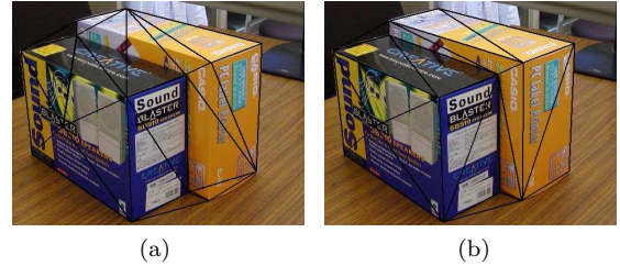
Figure 6: (a) Initial triangulation (31 edges). (b) Optimized triangulation (100% correct, 3 rounds, 3.15 sec).
