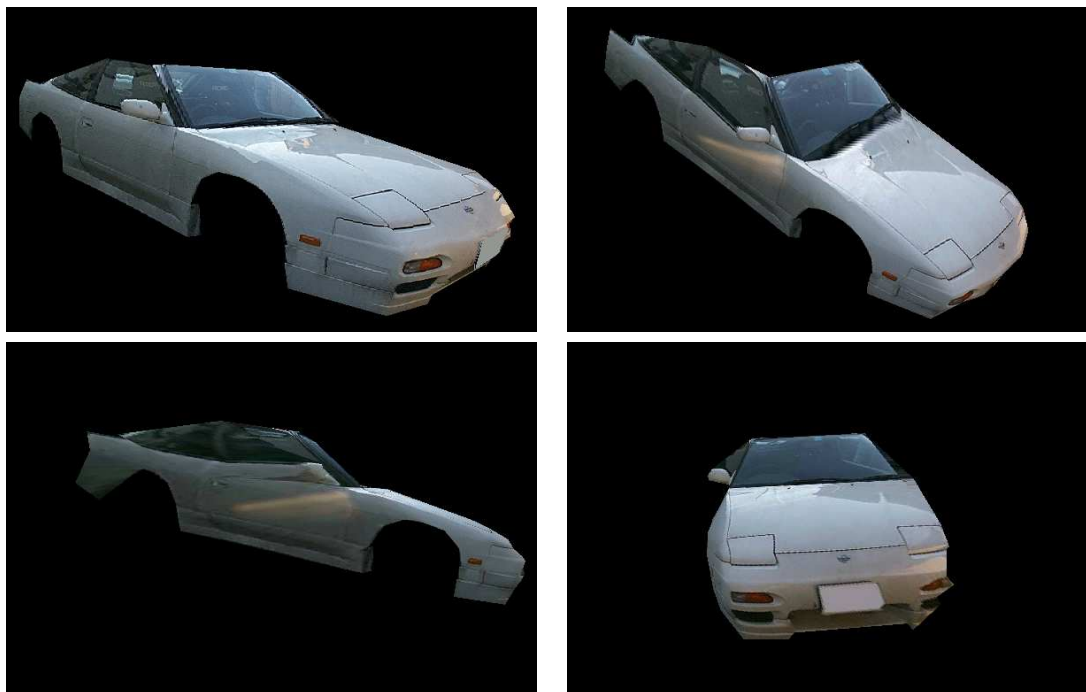
Figure 9: The reconstructed and texture-mapped 3-D shape: the finite motion approach (above); the optical flow approach (below).
