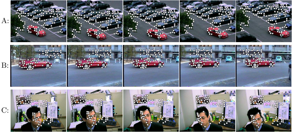
Fig. 5. Three video sequences and successfully tracked feature points
