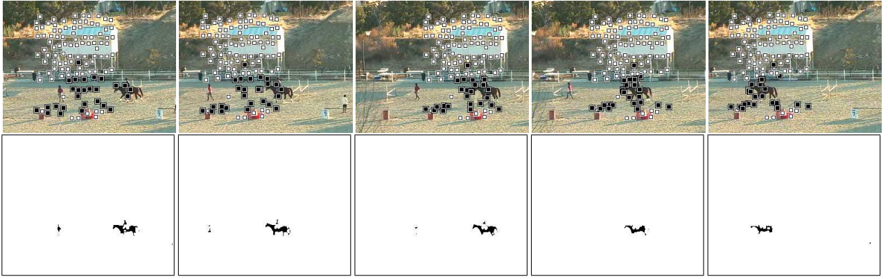
Figure 3 Five decimated frames from a 100 frame sequence (above) and detected moving objects (below).
